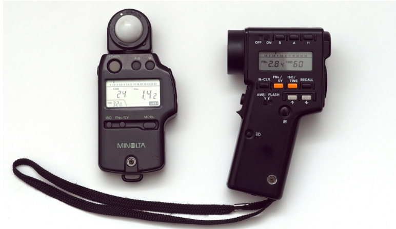
Figure 21: Left: an incident meter, notice the white ball. Right: a reflective (spot) meter used as a telescope to get a measurement. Some meters combine both measurement into one device.
